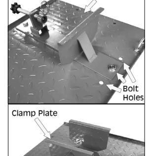
4. Attach the ramp to the rear side of the platform as shown.
